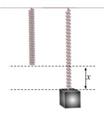
A force must be applied to displace the spring from the system of equilibrium position. An internal force is exerted when the spring is displaced directed back toward the system's equilibrium position (Restoring force).
