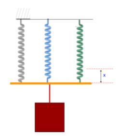
When connecting springs in parallel, the total displacement equals the displacement of the individual spring.
